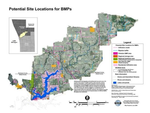
"Best management practices" – or BMPs – are stormwater control measures that slow, retain or absorb nonpoint source pollutants associated with runoff. When placed in these priority areas throughout the watershed, these BMPs can help control stormwater pollution in our local waterways.
